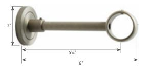
METAL WALL/CEILING BRACKET DX141 Bracket projection may be reduced from 5¼" max to 2 5/8" min Custom Bracket Cut DB900
