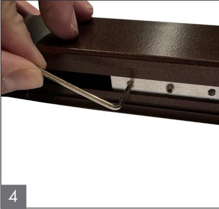
Loosen screws of already installed splice connector near the center splice. Slide splice connector over to cover both rods equally and tighten all screws to lock rods into place (center hole is intentionally left open to accommodate a center bracket).
